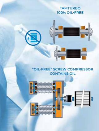
Thanks to the AMBs, the rotor and turbo impellers of the compressor levitate in air and do not come into contact with anything. With no metal to metal contact, the compressor does not wear or need any lubrication. Tamturbo compressors are directly driven variable speed drive (VSD) compressors without gear box or couplings. VSDs are used to change the motor speed to match the compressor output to air demand.
